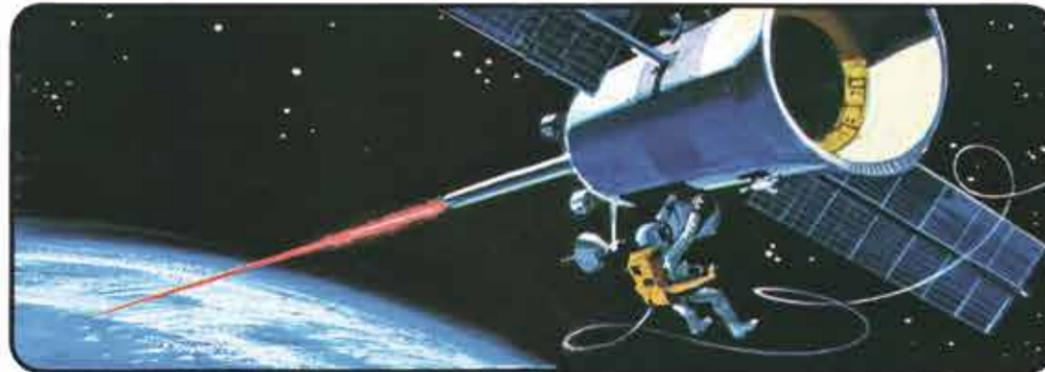
▲ This satellite, shown being serviced by an astronaut-engineer, has a laser to measure the small movements in the Earth's crust which are early indicators of earthquakes. This one is focused on a reflector embedded in the ground near the
