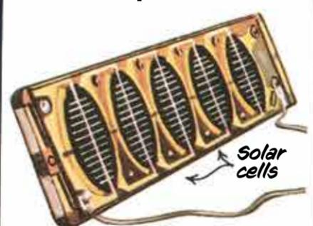
Solar cells are flat panes of silicon material which convert the energy in sunlight into electricity. A panel like this could help charge the car.
