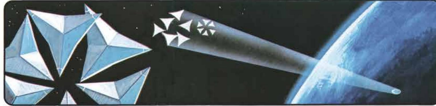
▲ These triangular satellites, each one 300 metres across, are in fact giant mirrors made of reflective aluminium foil. They are designed to focus sunlight onto the nightside of the world. The mirrors' beams could be switched from
