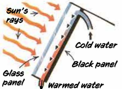
Solar panels on the roof help heat water for the house, saving energy. The panels take the chill off the mains water before an ordinary immersion heater boosts it to hot-bath temperatures.
