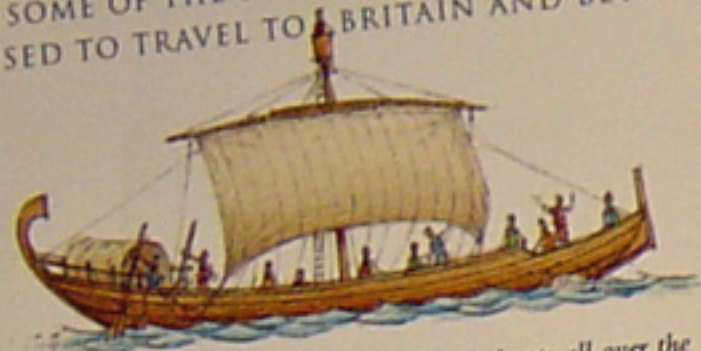
A trading vessel of the type used by merchants all over the Mediterranean. It was steered by large paddles at the stern.
