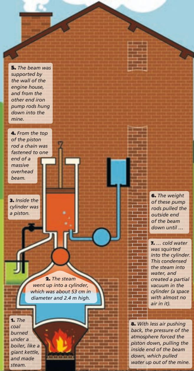
5. The beam was supported by the wall of the engine house, and from the other end iron pump rods hung down into the mine.
